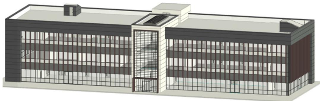
The Workers Building is to be formed with a combination of flat cladding panels in complimentary colours as per the palette and images below.
